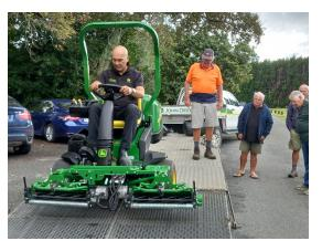
hydraulic points so it is really the lifter only that is hydraulically driven. The cruise control setting should reduce the diesel consumption and it should also operate more quietly. It also has ridged stainless steel rollers as opposed to the wooden ones on the old mower. The costs of these mowers have already risen across the board and the 2500 hydraulic version is much more expensive now. We will be placing the old
